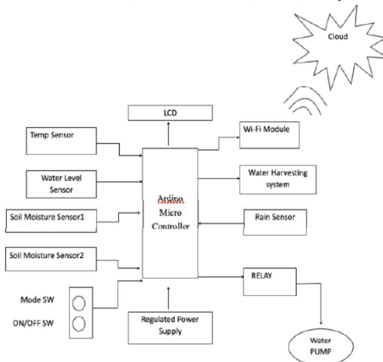
Figure 4. Block Diagram of Irrigation System Using Wireless Sensor Network (Pasha, et al., 2020)
